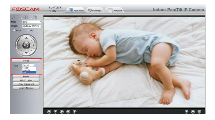
There are other buttons between the Preset points and Cruise track, you can use these buttons to adjust the order of preset points or add/delete one preset points in one cruise track.
